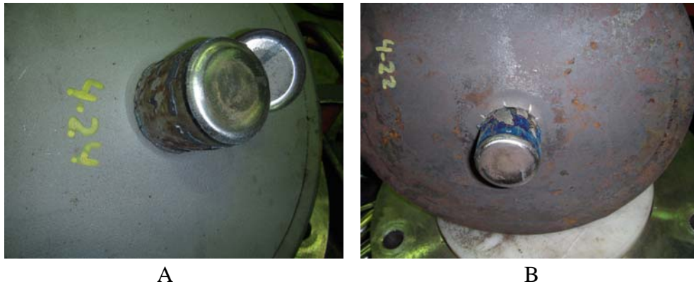
Figure 9. Punctured “super-tough” A710 Grade B (A) and A709 HPS100 (B) steel plates
