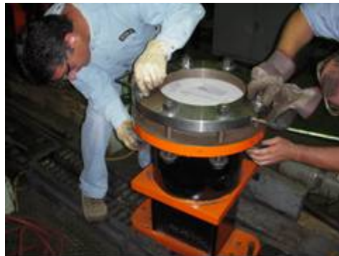
Figure 7. Assembly of the plate into holder for a penetration test
