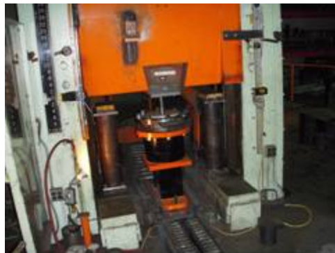
Figure 8. Placement of the plate into press prior to penetration test
