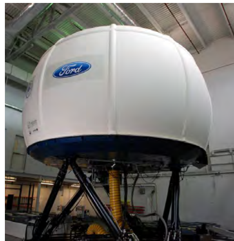
Figure 2- Exterior of VIRTTEX driving simulator
