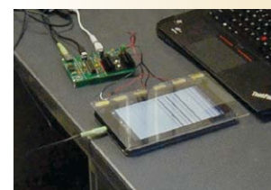
Haptic interface prototype that incorporates off-the-shelf e-book reader hardware.
