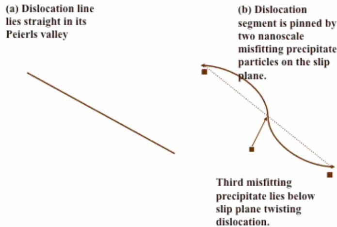
Figure 2 A misfit center lying above or below a dislocation line segment twists it partially out of its Peierls valley reducing the flow stress
