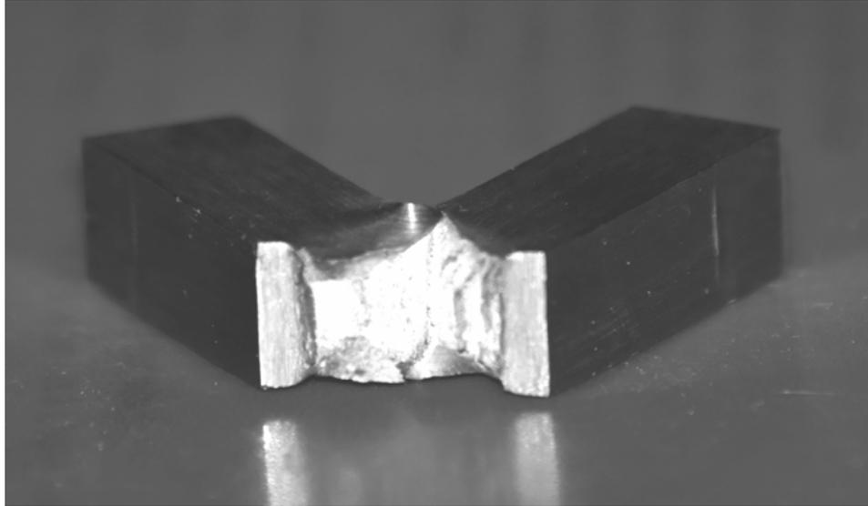
Figure 7. Charpy specimen of A710 Grade B with 0.10 % Ti tested at  $-40^{\circ}\text{C}$ . The specimen stopped Charpy hammer without fully fracturing. Fracture surface is completely ductile
