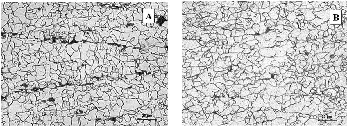
*Figure 4 Optical micrographs of (A) A710 B with 0.03 wt pct Ti and (B) Ti-modified A710 B with 0.10 wt pct Ti*
